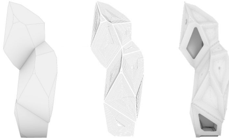
Fig. 20. Texturization and production of holes in component
